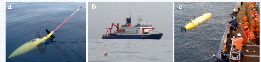
(a) Deployment of autonomous glider, (b) surfacing glider with the research icebreaker Polarstern in the background, (c) deployment of AUV (autonomous underwater vehicle) equipped with thruster propulsion (photographs Agnieszka Beszczyńska-Möller).
