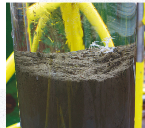
The picture of sediment core with benthic organisms (soft corals) that may actively mix bottom sediments (photograph A. Zaborska).
